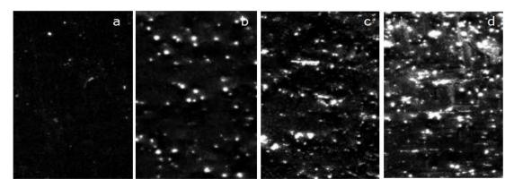
Figure 3. Dispersion images of NR based vulcanizates (a) NR, b) NR-HCF-1, c) NR-HCF-3, d) NR-HCF-5
