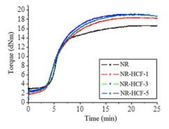
Figure 2. Rheometer curves of NR and NR/HCF based rubber compounds at 150 °C
