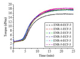
Figure 4. Rheometer curves of NR/ENR based rubber compounds at 150 °C
