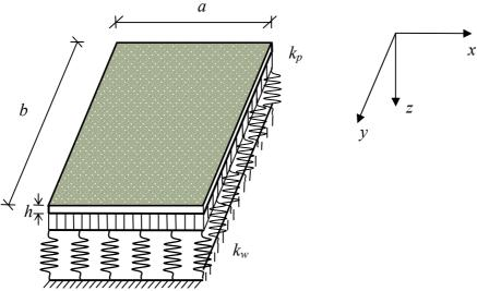
Fig. 1. Coordinate system and continuum model of an embedded single-layered graphene sheet
