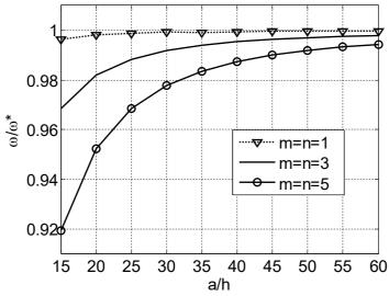
Fig. 2. Variation of the frequency ratio (with rotary inertia/without rotary inertia) with respect to a/h and mod number ( $K_w = K_G = 10$ , a = b, l = h)
