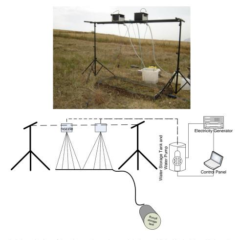
Figure 2. Schematic view of the BSTF1. Above, the actual device established in the lab and below, the general structure of the BSTF1 Şekil 3. BSTF1'in şematik görünümü
