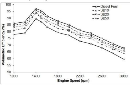
Fig. 5.Comparison of volumetric efficiency results
