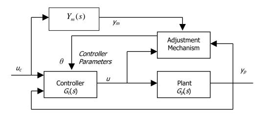
Figure 2: Block diagram of an adaptive control.
