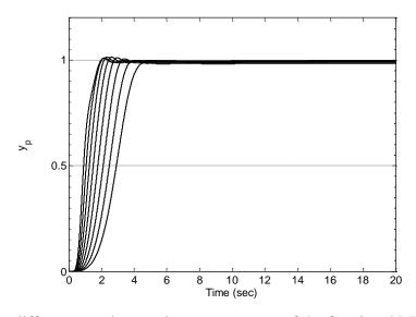
**Figure 8:** For different *K* values, unit step responses of the fractional MRAPI<sup> $\lambda$ </sup>D<sup> $\mu$ </sup> control.
