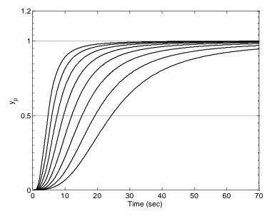
Figure 11: For different *K* values, unit step responses of the MRAPID control.
