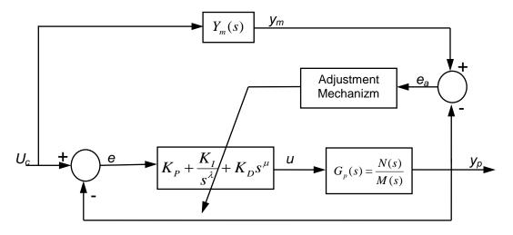
**Figure 3:** Block diagram of model reference adaptive  $PI^{\lambda}D^{\mu}$ .
