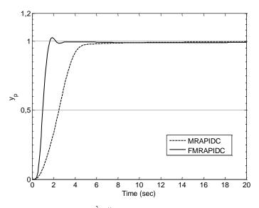
**Figure 6:** For fractional MRAPI $^{\lambda}D^{\mu}$  and MRAPID control the unit step responses.
