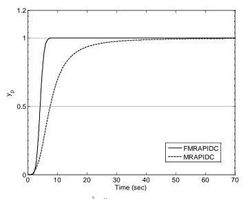
**Figure 10:** For fractional MRAPI $^{\lambda}D^{\mu}$  and MRAPID control the unit step responses.
