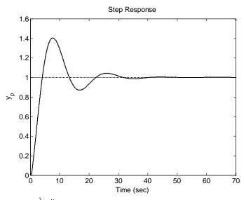
**Figure 9:** For  $PI^{\lambda}D^{\mu}$  controller, the unit step response of control system.
