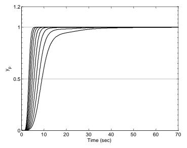
**Figure 12:** For different *K* values, unit step responses of the fractional MRAPI<sup> $\lambda$ </sup>D<sup> $\mu$ </sup> control.
