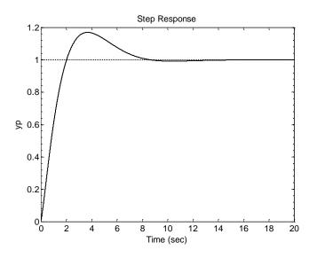
**Figure 5:** The unit step response of control system for  $PI^{\lambda}D^{\mu}$  controller.
