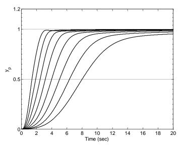
Figure 7: For different *K* values, unit step responses of the MRAPID control.
