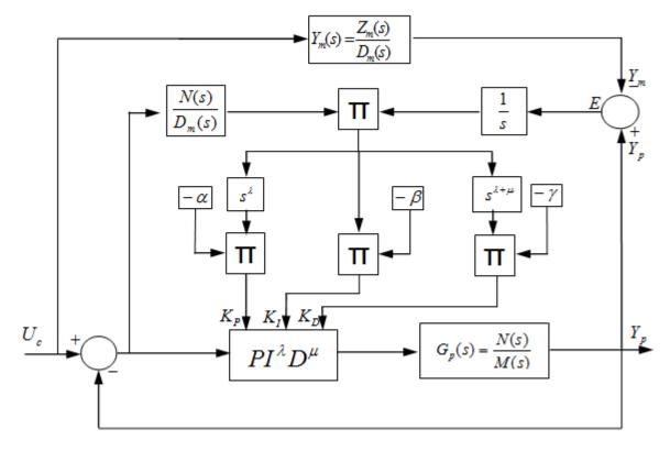
**Figure 4:** The control system block diagram of fractional MRACPI $^{\lambda}D^{\mu}$  control.
