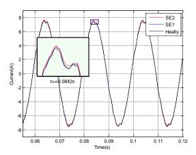
Figure 5: Current signals of LSPMSM for healthy and fault status
