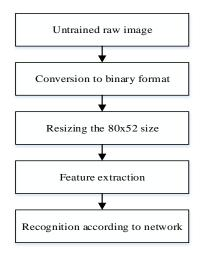
Figure 3: System Algorithm
