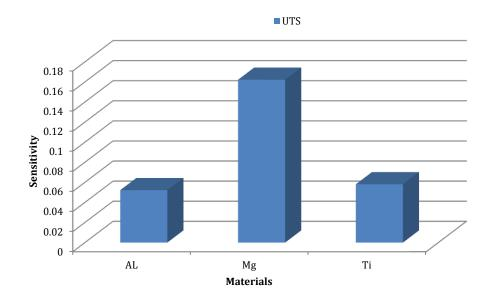
Fig. 3: Sensitivity of the materials on tensile strength
