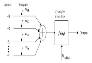
Fig. 1: Basic elements of an artificial neuron.
