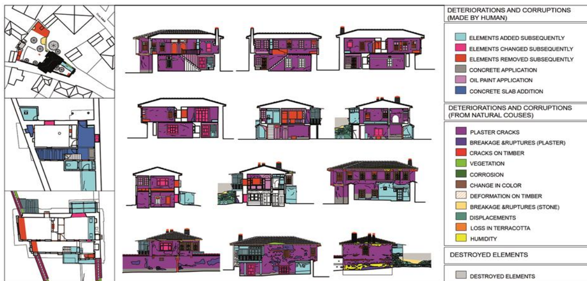
Figure 5. Deteriorations and corruptions of the mansion
