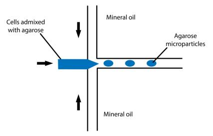
Figure 4: Schematic diagram of microfluidic device to produce bacteria with agarose hydrogel. Figure adapted from (25).
