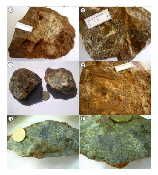
**Figure 6.** Photographs showing macro ore minerals from the Gürkuyu Sb mineralization (a), (b), (c) and (d) photographs showing mainly antimuan okr with skeletal texture and radial antimony (e), (f) antimony, pyrite, orpiment and realgar.
