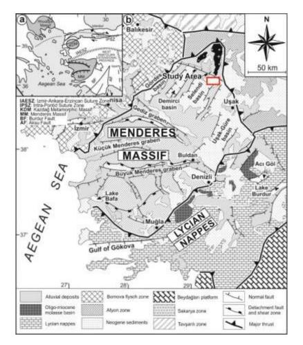
Figure 2. Tectonical map of the Gürkuyu Sb mineralization
