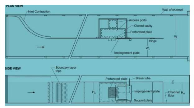
Figure 1. Overview of perforated plate-cavity system in large scale water channel.
