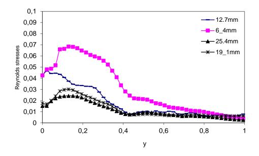
Figure 8. Reynolds stress for each perforated plate along spanwise axis
