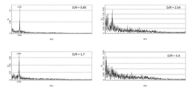
Figure 9. Pressure spectra for each perforated plate. Impingement length to momentum thickness ratio is  $L/\theta = 17.75$
