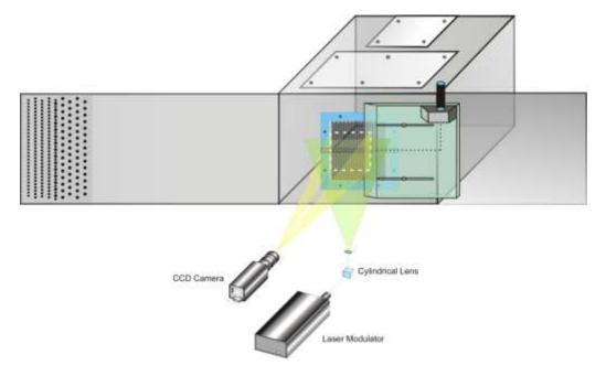
Figure 3. 3D view of cavity and laser orientation
