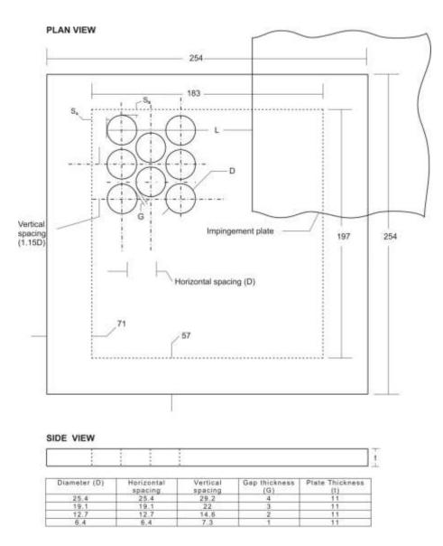
Figure 2. Dimensions of Perforated plates. (All dimensions are in mm.)
