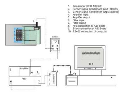
Figure 4. Pressure signal lines from transducer to host microcomputer.
