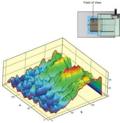
Figure 6. Three dimensional contour plot of cross spectral density  $S_u$  for the smallest diameter holes  $D/\theta = 0.85$ .
