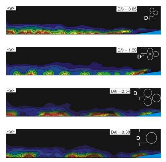
Figure 5. Spanwise velocity contours for each perforated plate
