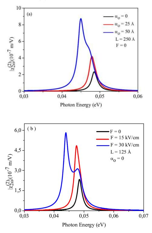
Fig. 3. Second Harmonic Generation (SHG) for an asymmetric parabolic quantum well as a function of the incident photon energy for three different values of (a)  $\alpha_0$ , (b) electric field.
