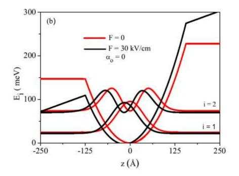
**Fig. 1.** The changes of the confinement potential profile, the ground and the first excited state energies and squared wave function corresponding to the two lowest energy levels considering two values of (a) ILF parameter, (b) electric field.
