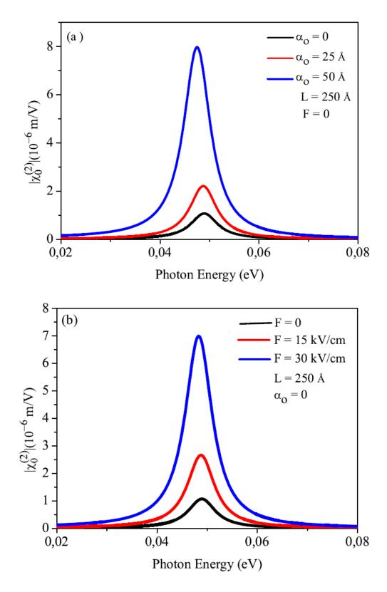
Fig. 2. The variations of the NOR coefficients as a function of the incident photon energy for three different values of (a)  $\alpha_0$ , (b) electric field.
