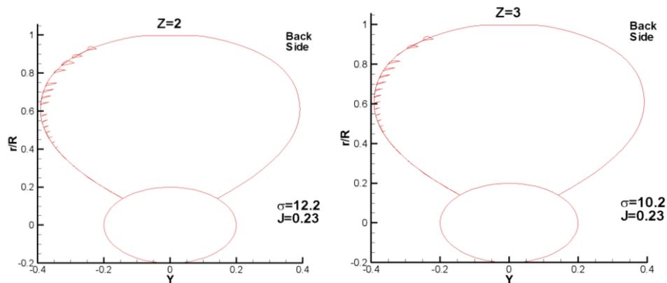
**Figure 3.** Comparison of cavity pattern of DTMB 4119 propeller
