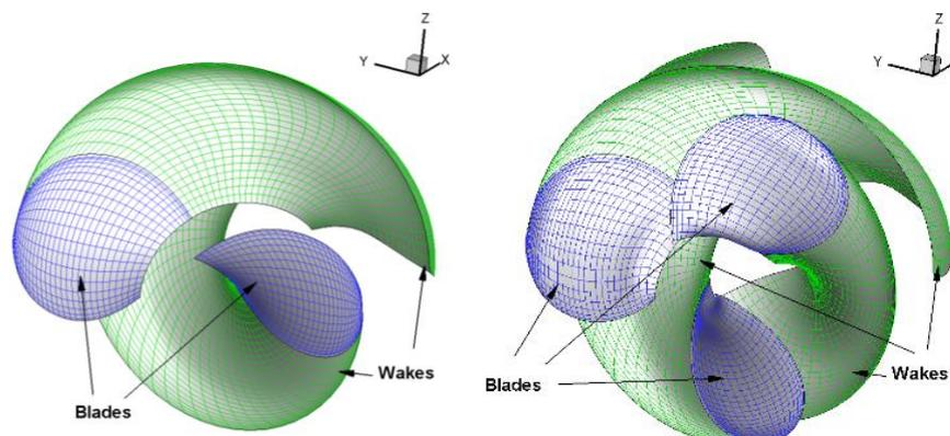
**Figure 2.** Perspective view of DTMB 4119 propeller blades and wakes
