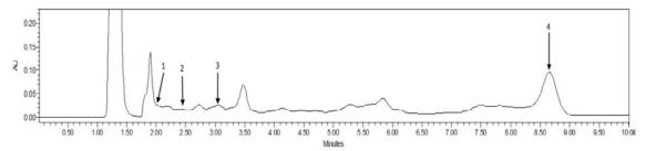
Figure 6. OLE MeOH extraction chromatogram 1. Hydroxytyrosol; 2. Tyrosol; 3. Verbascoside; 4. Oleuropein
