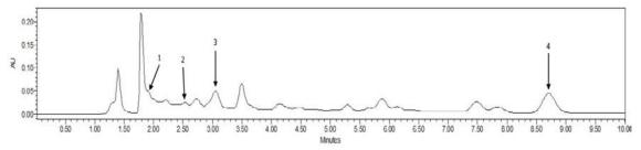
Figure 5. OLE MeOH/water extraction chromatogram 1. Hydroxytyrosol; 2. Tyrosol; 3. Verbascoside; 4. Oleuropein
