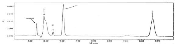
Figure 3. Chromatogram at 280 nm wawelength of the external standarts 1. Hydroxytyrosol; 2. Tyrosol; 3. Verbascoside; 4. Oleuropein
