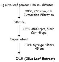
Figure 2. The schema of olive leaf extraction.
