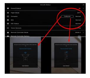
Fig. 5. Calibrating the compass of the unmanned aerial vehicle
