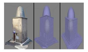
Fig. 11. Solid Model Creation - Build Mesh - Triangle Model (Build Mesh)
