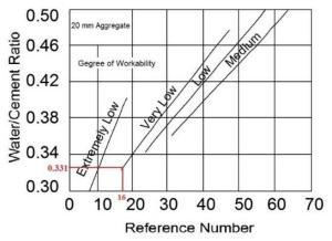
Figure 3: Relation between water/cement ratio and reference number for 200 mm maximum size aggregates [14].
