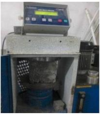
Figure 5: Compressive strength test of the first sample.
