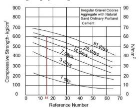
Figure 2: Graph of obtaining reference number [14]. According to graph in Figure 2, Reference Number is equal to 16.
