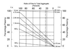
Figure 4: Combining coarse aggregate (C.A) and fine aggregate (F.A).
