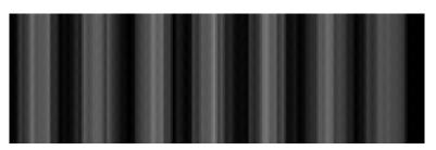
Figure 4- Modeled Interferogram Interference Signal
