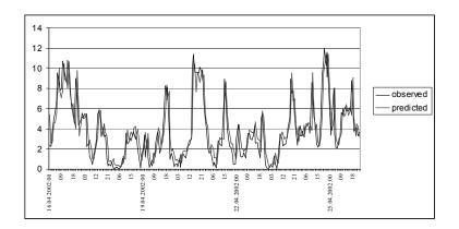
Figure 4.5 - Observed and predicted wind speed (m/s) values for hourly time series test data
