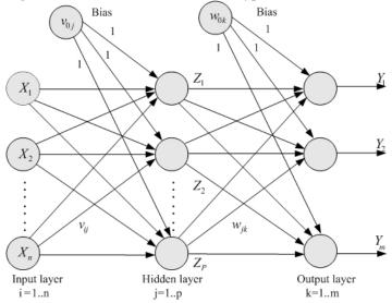
Figure 3.1- Structure of multi layer perceptron neural network
