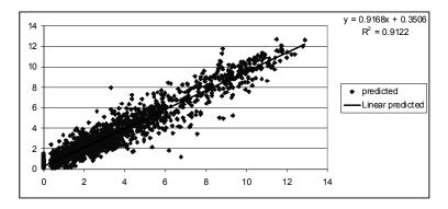
Figure 4.8 - Regression of predicted-observed wind speed (m/s) values for ten minutes time
