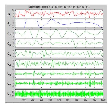
Figure 4- Application of db4 wavelet transform to EEG data of s1
