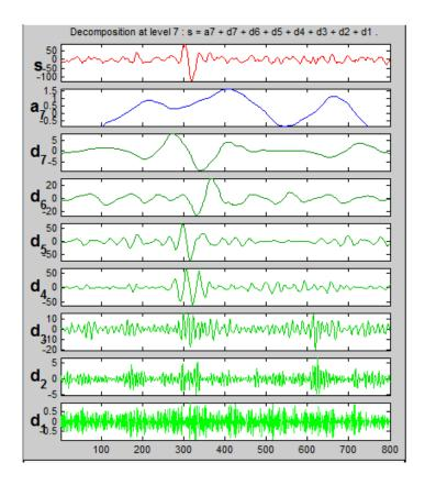
Figure 6- Application of db4 wavelet transform to EEG data of s2
