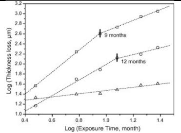
Figure 3. Bilogarithmic plots of data points from Figure 2.  $\Box$ : samples exposed at 95m station far from the sea line;  $\Delta$ : samples exposed at 375m station far from the sea line;  $\circ$ : samples exposed at industrial environment [8]
