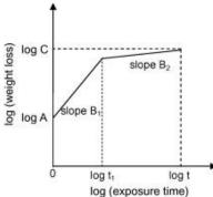
Figure 4. Schematic diagram of the variation of the thickness loss of mild steel in the marine atmosphere with time in log-log coordinate
