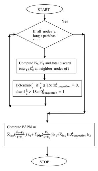
Fig. 4. Flow Diagram for computing routing metric of a path
