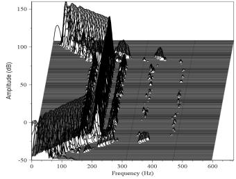
Figure 3: Waterfall graph of PMSM under 18% demagnetization fault.
