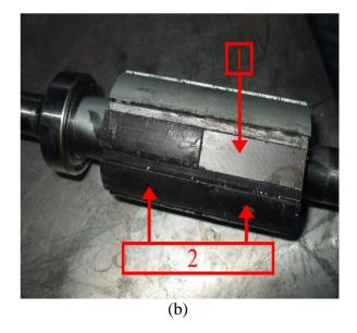
*Figure 1:* (a) *Experimental test rig (1: PMSM, 2: Brake, 3: Brake controller, 4: Power supply, 5: Motor controller, 6: Data acquisition board). (b) Damaged magnets of surface-mounted PMSM (1: Removed Magnet, 2: Thermally demagnetizated magnets).*
