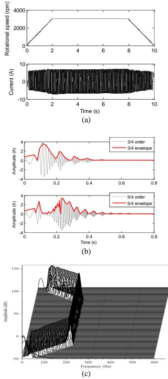
*Figure 2:* GOT results for healthy PMSM with speed profile 0-3000-0 r/min. ( a) Rotational speed and stator current. (b) Tracked 3/4 and 5/4 orders and corresponding envelopes of stator current. (c) Waterfall graph of the tracked orders.
