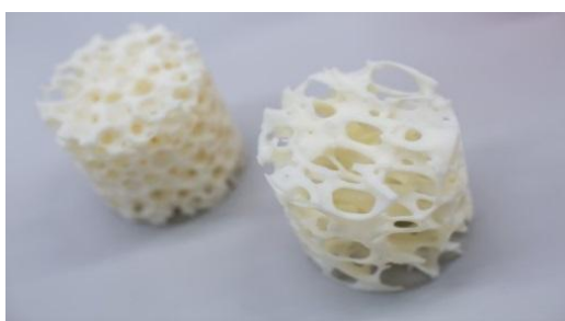
Figure 17. The graphitic nano carbon created by the PlasCarb technology has been tested by Abalonyx as reinforcement to bioglass. This material is used for the generation of transplantable bone tissue scaffolds [151].
