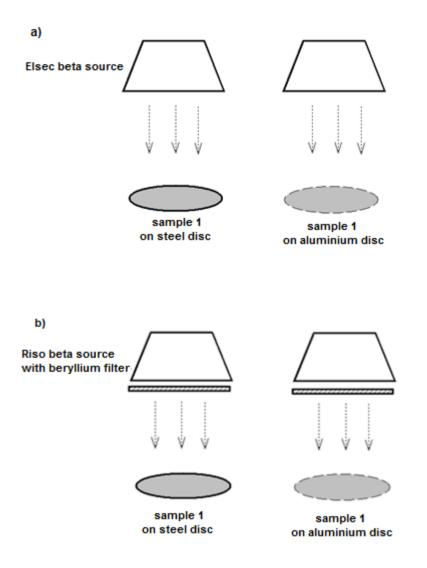
FIGURE 2. Three different mineral compositions were experimented with two different laboratory beta sources; one is the Elsec beta source and the other is the Riso beta source with beryllium filter. Three different samples were experimented, sample1: coarse grain quartz, sample2: fine grain feldspar, sample3: fine grain pottery.
