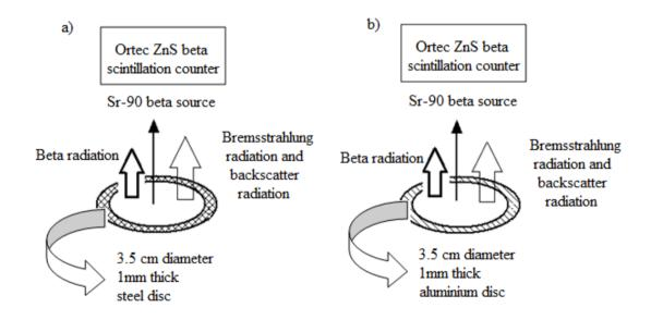
FIGURE 1. With this experimental configuration, the Ortec ZnS beta scintillation counter was also used to determine backscatter and bremsstrahlung radiation affects. Table 2 summarizes the results of this experiment. Plexiglas is not defined in this figure.
