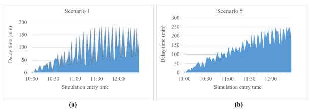
Figure 5: (a) Delay distribution of scenario 1 ( $\alpha$ =15°); (b) Delay distribution of scenario 5 ( $\alpha$ =15°)
