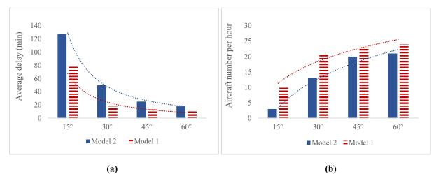
Figure 7: (a) Average delay time for different angles; (b) Capacity for different angles
