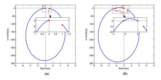
**Figure 3.** The Popov plot of the  $W(j\omega)$  (a) the case of  $k_i \leq (b/m)k_p$  (b) the case of  $k_i > (b/m)k_p$ .
