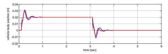
**Figure 18.** The closed loop system response. Road profile in black line, nonlinear PI controller response in red line, fixed-gain PI controller response in blue line.
