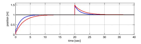
**Figure 8.** The output disturbance rejection response of the nonlinear PI and fixed-gain PI control system. Nonlinear PI controller response in blue line, PI controller response in red line, reference in black line.
