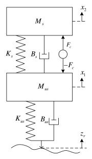
Figure 13. Double mass-spring-damper model for active suspension system [22].
