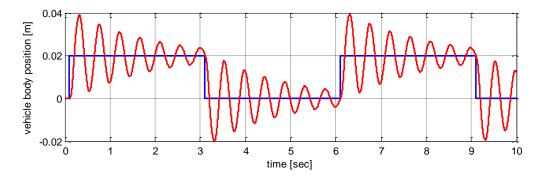
**Figure 17.** The open loop system response. Road profile in blue line, system response in red line.
