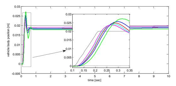
**Figure 23.** The controller performance for different parameters. Road profile in black line,  $\alpha$ =0.1,  $\gamma$  =2 in cyan line,  $\alpha$ =1,  $\gamma$  =2 in blue line,  $\alpha$ =0.5,  $\gamma$ =1 in green line,  $\alpha$ =0.5,  $\gamma$  =3 in magenta line, nominal values in red line.
