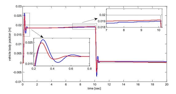
**Figure 22.** The closed loop system response. Road profile in black line, nonlinear PI controller response in red line, fixed-gain PI controller response in blue line.
