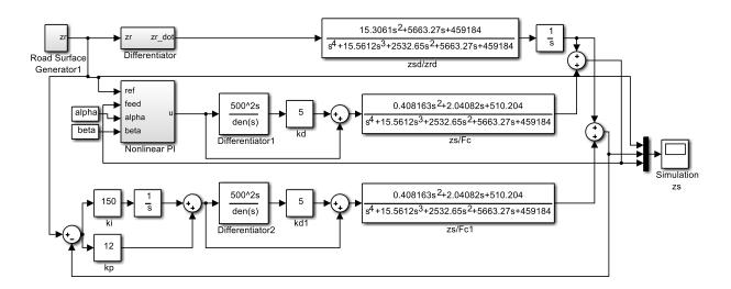
**Figure 16.** Simulation diagram constructed in Matlab/Simulink® for active suspension system. In simulations, road profile a square wave signal with a frequency of 0.1667 Hz and an amplitude of 0.02 is applied as the reference signal. In Figure 17, open loop system response is presented. As it is revealed in the figure, open loop system with no suppression ability has vibrations with large amplitudes.
