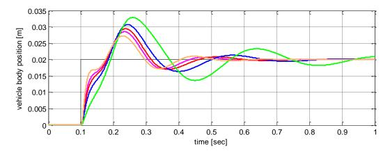
**Figure 19.** The controller performance for different parameters. Road profile in black line,  $\alpha$ =0.1,  $\gamma$  =2 in magenta line,  $\alpha$ =1,  $\gamma$  =2 in blue line,  $\alpha$ =0.5,  $\gamma$  =1 in green line,  $\alpha$ =0.5,  $\gamma$  =3 in orange line, nominal values in red line.
