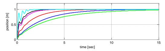
**Figure 11.** The controller performance for different  $\gamma$  parameters. Fixed-gain PI controller response in blue line,  $\gamma=1$  in green line,  $\gamma=2$  in red line,  $\gamma=4$  in magenta line,  $\gamma=5$  in black line,  $\gamma=10$  in cyan line ( $\alpha=0.4$  and  $\beta=1$ ).
