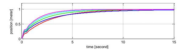
**Figure 9.** The controller performance for different  $\alpha$  parameters. Fixed-gain PI controller response in red line,  $\alpha=1.5$  in blue line,  $\alpha=1$  in green line,  $\alpha=0.5$  in cyan line,  $\alpha=1.5$  in magenta line ( $\beta=1$  and  $\gamma=2$ ).
