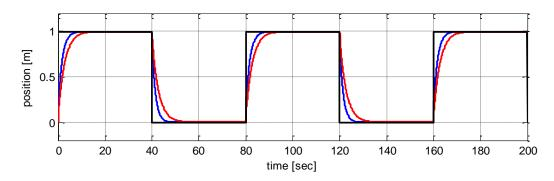
**Figure 6.** System response for nonlinear and fixed-gain PI controllers. Nonlinear PI controller response in blue line, fixed-gain PI controller response in red line, reference in black line.
