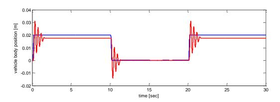
Figure 21. The open loop system response. Road profile in blue line, system response in red line.
