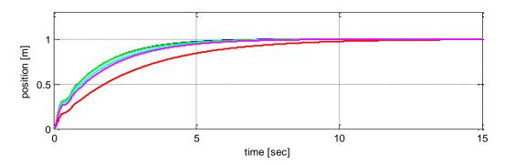
**Figure 10.** The controller performance for different β parameters. Fixed-gain PI controller response in red line,  $\beta = 100$  in blue line,  $\beta = 10$  in green line,  $\beta = 1$  in cyan line,  $\beta = 0.1$  in magenta line ( $\alpha = 0.5$  and  $\gamma = 2$ ).
