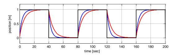
**Figure 12.** System responses for b=7.5 and k=900. Nonlinear PI controller response in blue line, fixed-gain PI controller response in red line, reference in black line.
