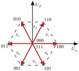
Figure 4. Space vector pulse width modulation vector diagram [7]
