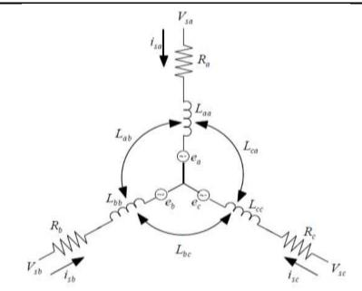
Figure 2. Three-phase equivalent circuit of a permanent magnet synchronous motor [3]
