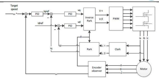
Figure 1. Speed control of permanent magnet brushless synchronous motor [3]
