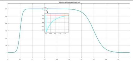
Figure 12. Asymmetric S-Curve speed reference and feedback (rpm)
