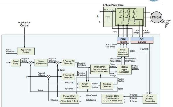
Figure 9. Permanent magnet brushless synchronous motor control algorithm
