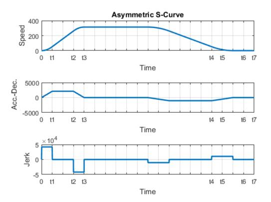
Figure 8. Asymmetric S-Curve speed profile
