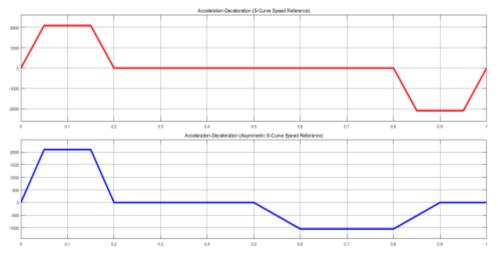
Figure 17. Acceleration-Deceleration graph according to reference speed profiles
