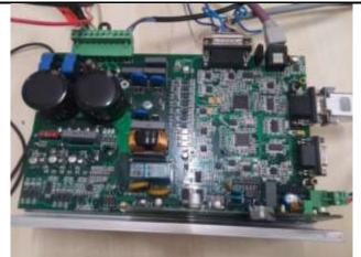
Figure 14. Control card with TMS320x28xxx microcontroller
