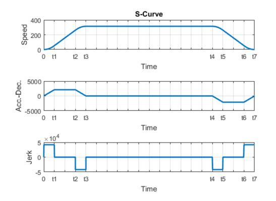
Figure 7. S-curve speed profile Jerk(J) is calculated and s-curve speed profile is created. Equation [18 and 19] is used for the S-curve speed profile [11].
