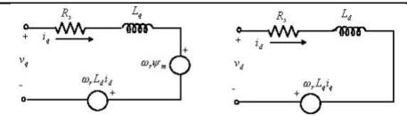
Figure 3. D-Q axis equivalent circuit of the permanent magnet synchronous motor [3]
