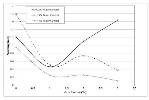
Figure 4. Jute content-Swelling behavior of the specimens.
