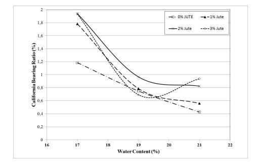
Figure 2. Water content-CBR behavior of the specimens.
