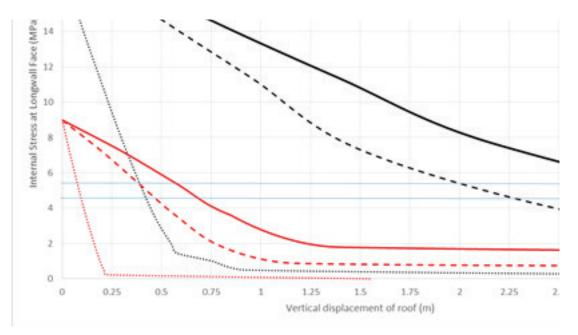
Figure 5. Ground response behavior for 400 and 800m depths and different face lengths
