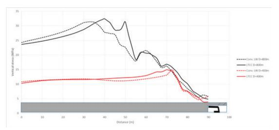
Figure 4. Vertical stress distribution along the mid-face for different depth and mining methods
