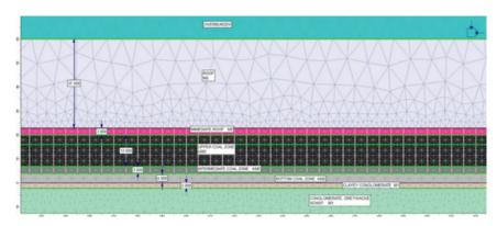
Figure 3. Zoomed view of coal seam numerical model with strata thicknesses and mesh for southern Soma coal mines
