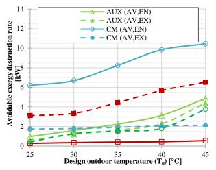
Figure 7. Influence of the approach temperature of GC on the endogenous and exogenous avoidable exergy destruction rates of the components belonging to PC at different  $T_0$ .
