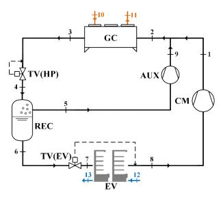
Figure 1. Schematic of a R744 refrigeration system with parallel compression economization (PC).
