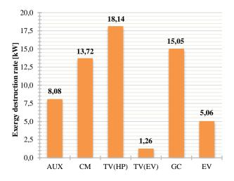
*Figure 2. Results of the conventional exergy analysis associated with PC* ( $T_0 = 40$  °*C*).
