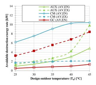
Figure 5. Influence of the design outdoor temperature (i.e. dead state temperature or  $T_0$ ) on the endogenous and exogenous avoidable exergy destruction rates of the components belonging to PC.
