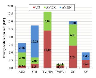
Figure 3. Results of the advanced exergy analysis associated with PC ( $T_0 = 40$  °C).
