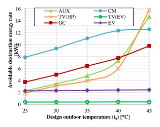
Figure 4. Influence of the design outdoor temperature (i.e. dead state temperature or  $T_0$ ) on the avoidable exergy destruction rates of the components belonging to PC.
