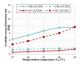
Figure 6. Influence of the increase by 10% of CM efficiency on the endogenous and exogenous avoidable exergy destruction rates of the components belonging to PC at different  $T_0$ .
