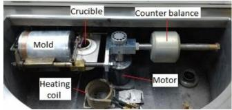
Fig. 3. Centrifugal casting machine and mold
