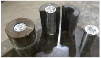
Fig. 1. Pre-samples and steel molds
