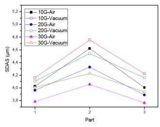
Fig. 12 SDASs of samples fabricated by D mold
