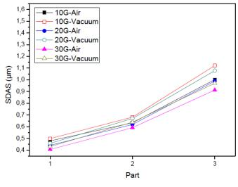
Fig. 9 SDASs of samples fabricated by A mold
