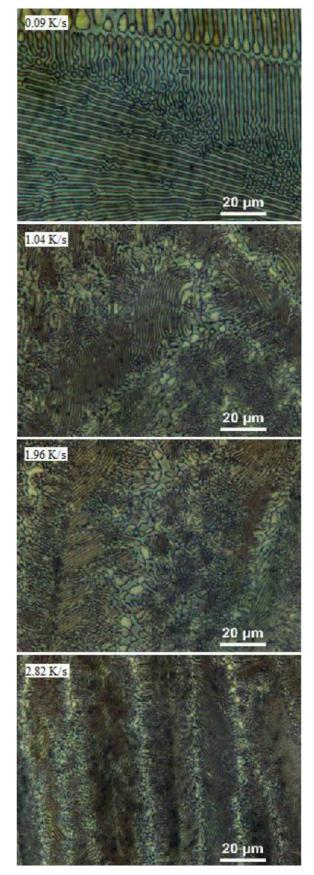
Fig. 7. Microstructures of samples fabricated in different cooling rates
