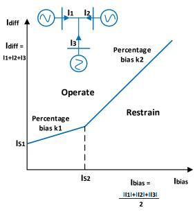
Figure 1. Dual Slope Bias Technique
