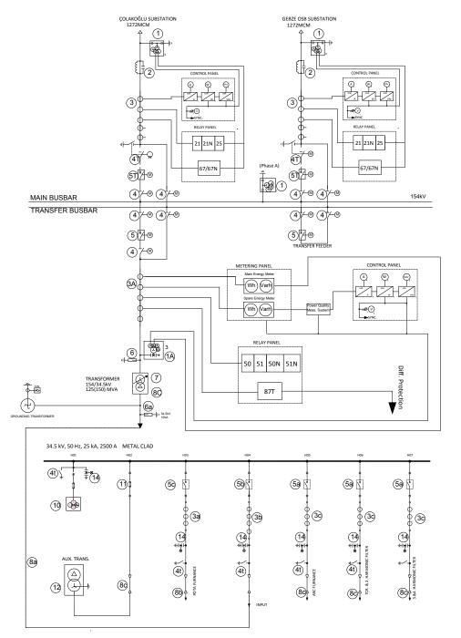
Figure 2. SKS Single Line Diagram [12]
