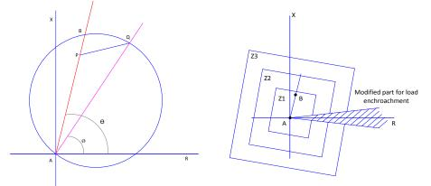
*Figure 6.* (*a*): Increased Arc Resistance Coverage [3]. (*b*)Relay Characteristic modification for the load encroachment.
