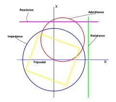
Figure 7. Zones of Protection in Distance Relaying
