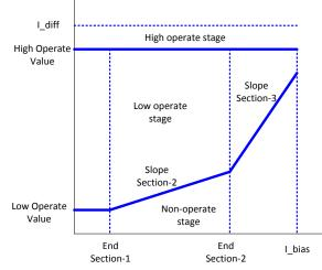
Figure 3. Operating characteristics of the DifP [6].
