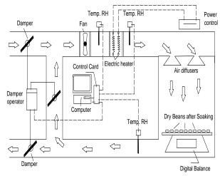
Figure 1. Drying system (Kurutma sistemi)
