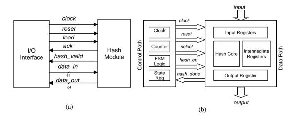
FIGURE 1. (a) Common I/O Interface (b) Hash Module separated in Control and Data paths
