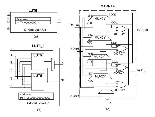
FIGURE 2. LUT5, LUT6\_2 and CARRY4 primitives in the Xilinx HDL library
