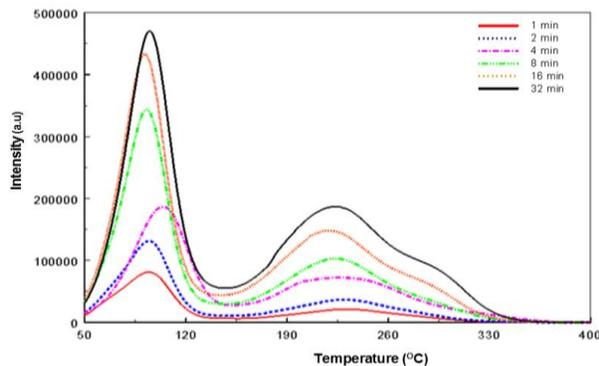
**Figure 2** Glow curves obtained by changing the irradiation time under a constant heating rate of 2 °C/s.
