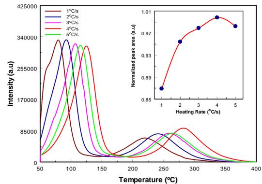
**Figure 4** Change of TL spectrum depending on heating rate under constant irradiation duration of 5 min.
