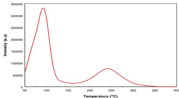
**Figure 1** Glow curve of the salt sample after X-ray irradiation for 15 min with a heating rate of 2 °C / s.
