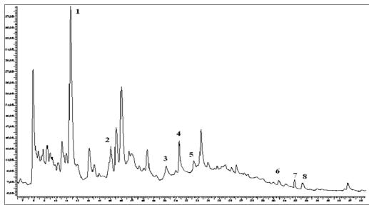
*Figure 3. HPLC chromatogram of the vinegar samples; chlorogenic acid (1), caffeic acid (2), p-coumaric acid (3), rutin (4), ferullic acid (5), quercetin (6), naringenin (7), kaempferol (8)*
