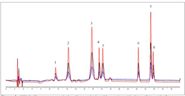
*Figure 2. HPLC Chromatogram of phenolic standards; chlorogenic acid (1), caffeic acid (2), p-coumaricacid (3), rutin (4), ferullic acid (5), quercetin (6), naringenin (7), kaempferol (8)*
