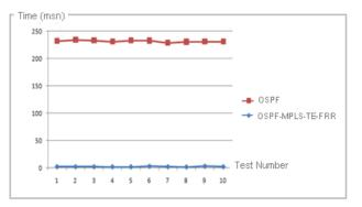
Fig.6. Comparative results of OSPF and OSPF-MPLS-TE-FRR's transition time
