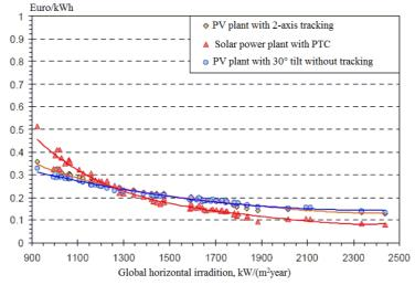
Figure 2. Cost price of the generated power energy on solar power plants
