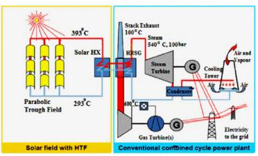
Figure 1. ISCC system schematic diagram
