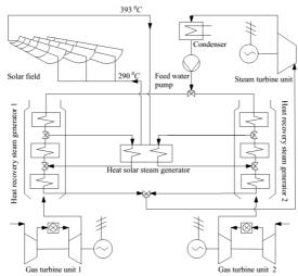
Figure 4. ISCC system schematic diagram based on PTC
