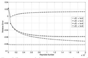
**Figure 7.** The amount of relative error comparison between the Tsal and Colebrook White equations.
