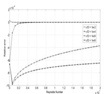
**Figure 3.** The amount of relative error comparison between the Zigrang- Sylvester and Colebrook White equations.
