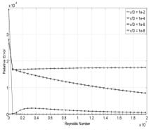
**Figure 4.** The amount of relative error comparison between the Buzzelli and Colebrook White equations.
