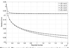
Figure 6. The amount of relative error comparison between the Altshul and Colebrook White equations.
