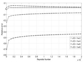
**Figure 5**. The amount of relative error comparison between the Wood and Colebrook White equations.
