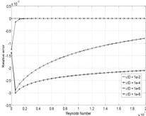
**Figure 2**. The amount of relative error comparison between the Serghides and Colebrook White equations.
