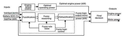
Figure 5. Fuzzy-based control system diagram [11]
