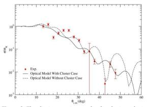
**Figure 2.** The elastic scattering angular distributions obtained with and without cluster case of <sup>17</sup>F by using the optical model. The experimental data have been taken from Zhang et al. (2012).
