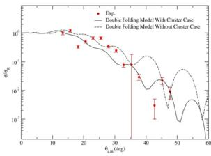
**Figure 3.** The elastic scattering angular distributions obtained with and without cluster case of <sup>17</sup>F by using the double folding model. The experimental data have been taken from Zhang et al. (2012).
