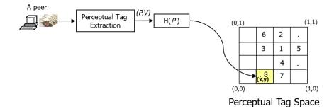
Figure 2. The proposed DHT based distributed perceptual tagging system as an analogue to the CAN design.
