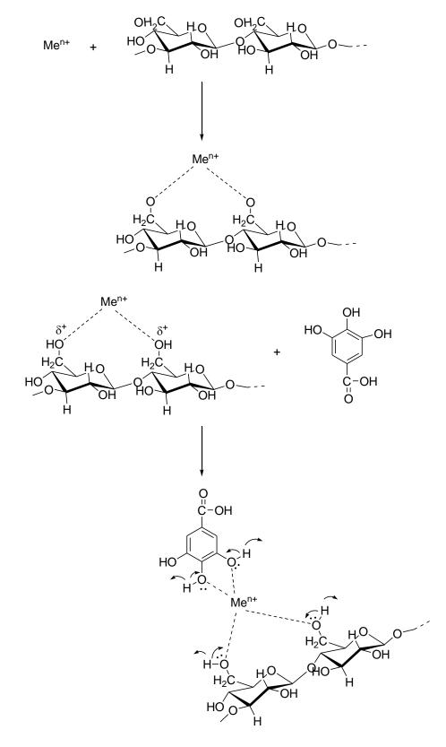
Figure 3. Proposed dyeing mechanism of linen (together mordanting.)
