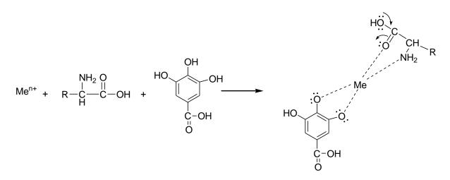
Figure 2. Proposed dyeing mechanism of wool (together mordanting.)
