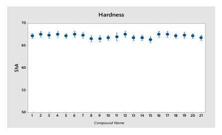
Figure 5. UV stabilizers effect on hardness
