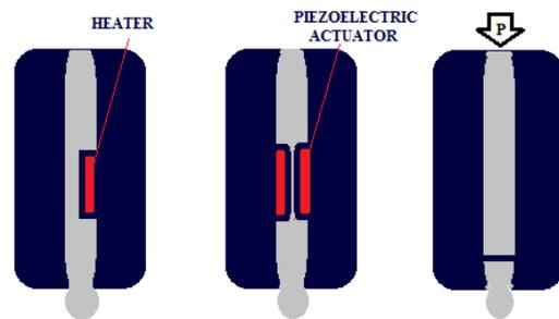
Figure 2. Schematic representation of inkjet printer methods.
