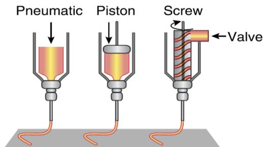
**Figure 3.** Microextrusion bioprinting systems [2].
