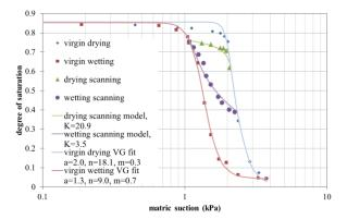
**Figure 14.** The proposed hysteresis model for a scanning loop (experimental data from [18]), the R<sup>2</sup> values for drying and wetting scanning curves are 0.979 and 0.934, respectively.
