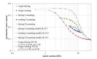
Figure 11. The proposed hysteresis model for scanning loop (experimental data from [17]), the R<sup>2</sup> values for drying I, wetting I and drying II scanning curves are 0.860, 0.908 and 0.901, respectively.
