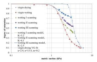
Figure 10. The proposed hysteresis model for wetting scanning curves (experimental data from [16]), the R<sup>2</sup> values for wetting I, wetting II and wetting III scanning curves are 0.958, 0.955 and 0.971, respectively.
