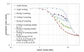
Figure 12. The proposed hysteresis model for scanning loop (experimental data from [17]), the R<sup>2</sup> values for wetting I, drying I and wetting II scanning curves are 0.929, 0.787 and 0.899, respectively.
