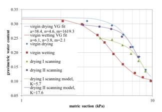
**Figure 5.** The proposed hysteresis model for drying scanning curves (experimental data from [11]), the R<sup>2</sup> values for drying I and drying II scanning curves are 0.970 and 0.992, respectively.
