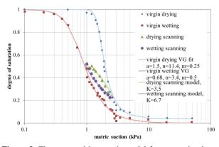
**Figure 3.** The proposed hysteresis model for a scanning loop (experimental data from [10]), the R<sup>2</sup> values for drying and wetting scanning curves are 0.890 and 0.917, respectively.
