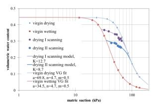
Figure 9. The proposed hysteresis model for drying scanning curves (experimental data from [15]), the R<sup>2</sup> values for drying I and drying II scanning curves are 0.935 and 0.822, respectively.
