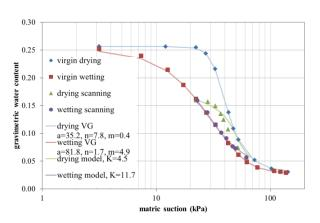
**Figure 4.** The proposed hysteresis model for a scanning loop (experimental data from [4]), the R<sup>2</sup> values for drying and wetting scanning curves are 0.924 and 0.993, respectively.
