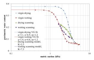
**Figure 7.** The proposed hysteresis model for a scanning loop (experimental data from [13]), the R<sup>2</sup> values for drying and wetting scanning curves are 0.980 and 0.991, respectively.
