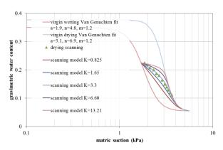
**Figure 15.** Sensitivity of scanning curves for parameter K (experimental data from [10]), the R<sup>2</sup> values for K=0.825, K=1.65, K=3.3, K=6.6 and K=13.21 are 0.548, 0.867, 0.980, 0.875 and 0.648, respectively.
