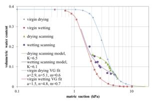
**Figure 8.** The proposed hysteresis model for a scanning loop (experimental data from [14]), the R<sup>2</sup> values for drying and wetting scanning curves are 0.956 and 0.923, respectively.
