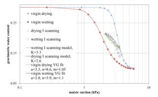
Figure 13. The proposed hysteresis model for scanning loop (experimental data from [17]), the R<sup>2</sup> values for wetting I and drying I scanning curves are 0.979 and 0.838, respectively.
