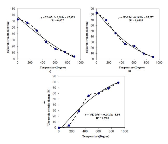
**Figure 2.** As the temperature rises, a) changes in flexural strength value for under 1 mm sieve aggregate b) changes in flexural strength value for under 2 mm sieve aggregate and c) the percentage change in the ultrasonic wave velocity for under 2 mm sieve aggregate.
