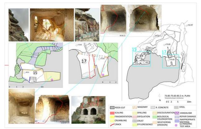
Figure 5. Damages and deteriorations in the space 15 and 17
