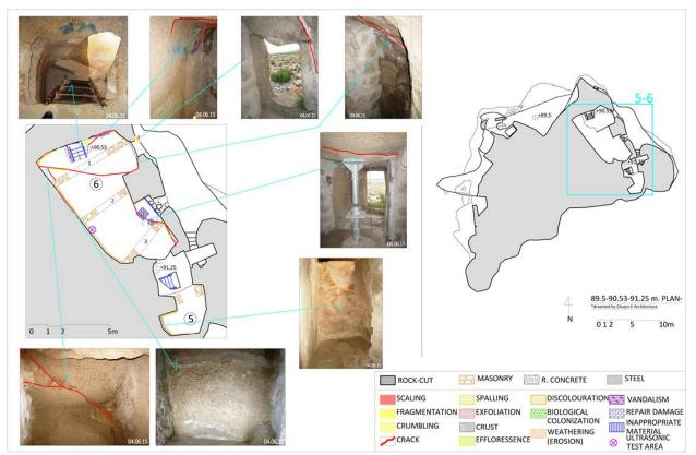
Figure 4. Damages and deteriorations in the space 5 and 6
