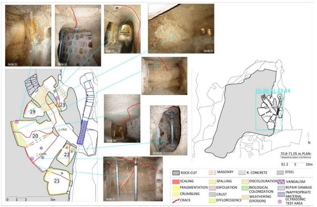
Figure 6. Damages and deteriorations in the space 19-20-21-22 and 23
