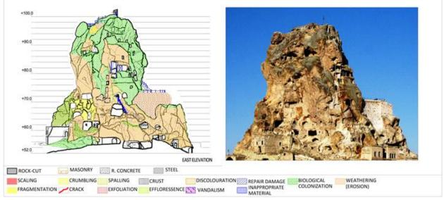
Figure 7. Damages and deteriorations on the east elevation
