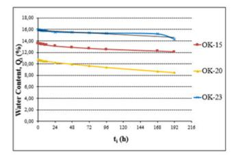
Figure 8. Water desorption of OK-15, OK-20 and OK-23
