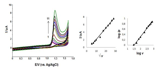
*Figure 4.* Influences of scan rate on the electrochemical oxidation peak current of 0.1 mM ofloxacin at the BDD electrode in phosphate buffer solution (pH 2.0) in presence of 1 mM SDS: (1) 30, (2) 50, (3) 75, (4) 100, (5) 200, (6) 300, (7) 400, (8) 500, (9) 600, (10) 700, (11) 800 mV/s. Inset: a plot of the peak current vs. the square root of scan rate and a plot of the logarithm of the peak current vs the logarithm of the scan rate for ofloxacin.
