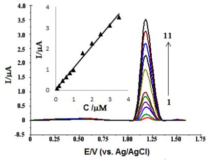
*Figure 8.* SW voltammograms in 0.1 M phosphate solution at pH 2.0 and presence of 1.0 mM SDS using a anodically pretreated BDD electrode at different of loxacin concentration levels: (1) 0.1, (2) 0.2, (3) 0.4, (4) 0.6, (5) 0.8, (6) 1.0, (7) 1.5, (8) 2.0, (9) 2.5, (10) 3.0 and (11) 3.5  $\mu$ M. (F = 100 Hz; A = 40 mV and  $\Delta E_s = 12$  mV). Inset: Analytical curve.
