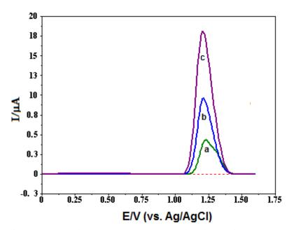
*Figure 7.* SW voltammograms in 0.1 M phosphate solution (pH 2.0) of 0.1 mM ofloxacin; (a) 0.1 mM ofloxacin, (b) 0.1 mM ofloxacin and 1.0 mM SDS (before optimization) (c) 0.1 mM ofloxacin and 1.0 mM SDS (after optimization)
