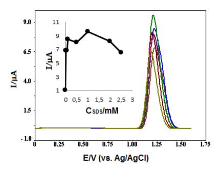
*Figure 2.* Square-Wave voltammograms of 0.1 mM ofloxacin at pH 2.0 of 0.1 M phosphate buffer on BDD electrode at different sodium dodecylsulfate concentration levels: (1) 0, (2) 0.01, (3) 0.05, (4) 0.1, (5) 0.5, (6) 1.0, (7) 2.0, (8) 2.5. (inset: Curve of the oxidation peak current on the SDS concentration).
