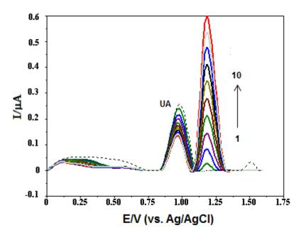
*Figure 10.* SW voltammograms for different concentrations of ofloxacin spiked in human urine sample in pH 2.0 (0.1 M phosphate buffer) and presence of 1 mM SDS. (1) 0.1, (2) 0.2, (3) 0.3, (4) 0.4, (5) 0.5, (6) 0.6, (7) 0.7, (8) 0.8, (9) 0.9, (10) 1.0.
