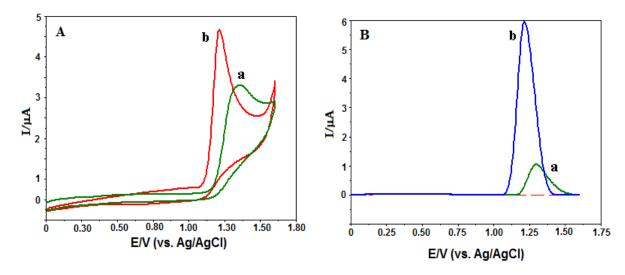
*Figure 3.* (A) The cyclic voltammograms at the BDD electrode in phosphate buffer solution (pH 2.0) of 0.1 mM ofloxacin, scan rate 0.1 Vs<sup>-1</sup>. (B) Square-wave voltammograms at the BDD electrode in phosphate buffer solution (pH 2.0) of 0.1 mM ofloxacin. (a; non-surfactant, b; with surfactant)
