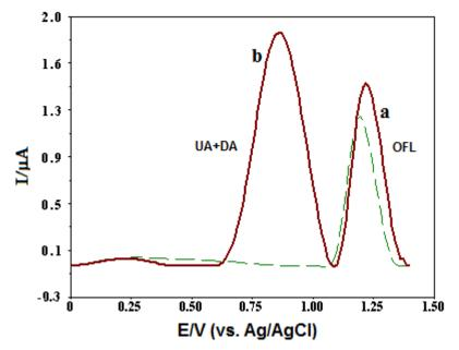
*Figure 9.* SW voltammograms in 0.1 M phosphate solution at pH 2.0 and presence of 1.0 mM SDS in mixture of (a) 0.001 mM ofloxacin and (b) 0.002 mM uric acid and dopamine. Dash line represent 0.001 mM ofloxacin at pH 2 phosphate solution.
