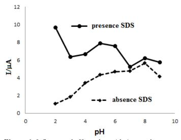
*Figure 6.* Influence of pH on the oxidation peak current of 0.1 mM ofloxacin in absence and presence SDS at BDD electrode in phosphate buffer (pH 2.0-9.0)
